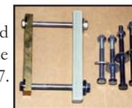
Brass-FRP mini-press only (with plated nuts, flat washers and bolts).
